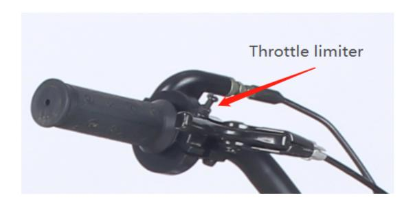
The throttle limiter is located on the right side of the handlebars. The speed limiter can be adjusted to Two-thirds of the normal speed.
