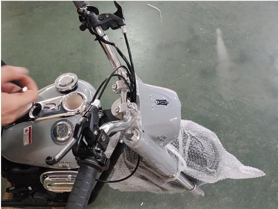
3. Adjust the brake, throttle handles, and tighten the bolts.
