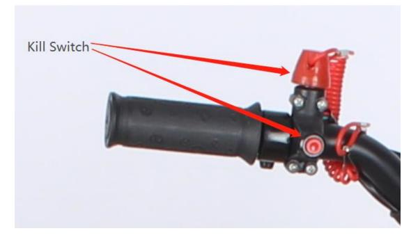
The emergency rope can be fastened to the rider in case there is an emergency. The vehicle will stop automatically when the rider pulls the rope.
