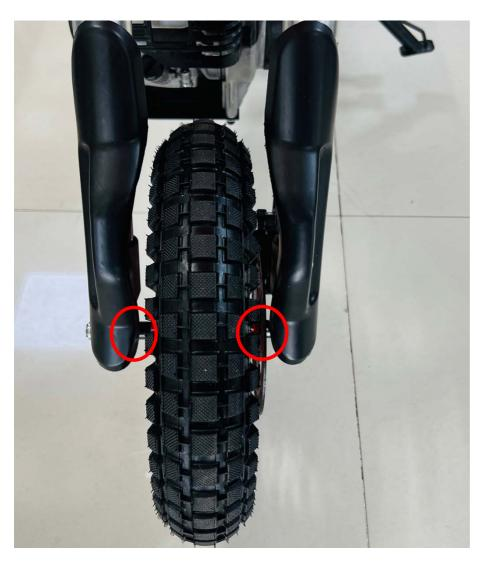
5. Install the front fender and number plate.
