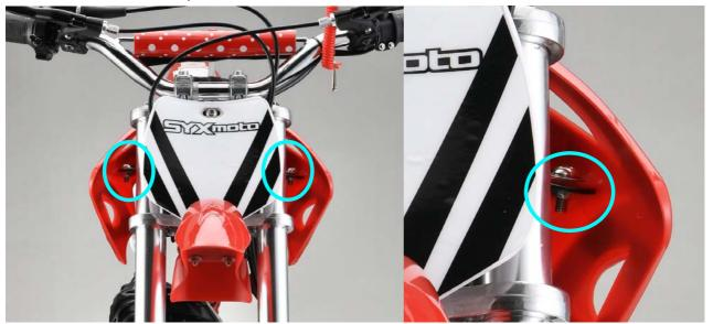
two screws on the front side panels connected to the fuel tank
