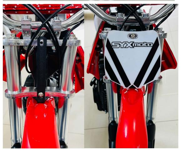
6. Secure the plastic cover with the included screws, and tight the bolts.
