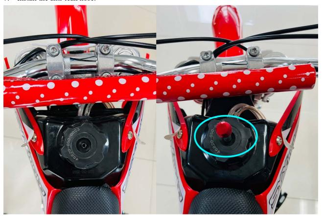
8. Adjust and tight the throttle and brake, make sure that the throttle limit screw does not interfere with the brake.
