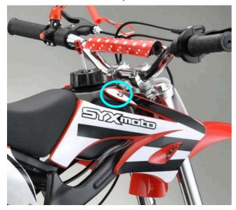
Two scres on the rear side panel connected to the frame
