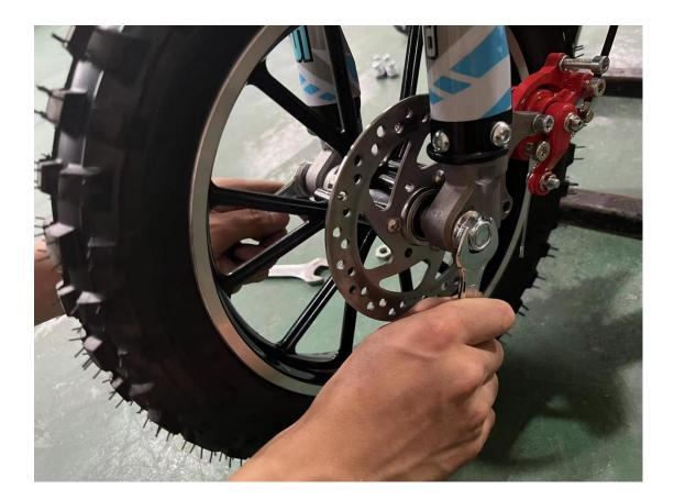
4. Remove the front brake caliper and install the front brake caliper.
