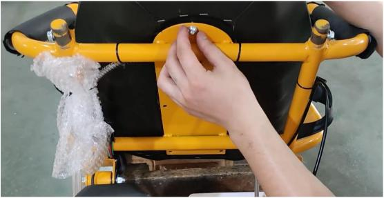
3. Install the seat belt and rear shock absorber, but do not tighten the bolts at this time.
