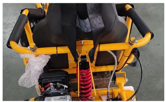
4. Loose the bolts and install the rear protection frame. Tighten the bolts.
