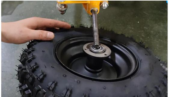
9. Install the steering wheel, and tighten the bolts.
