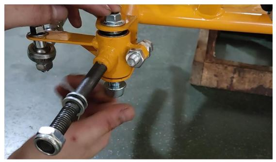
8. Install the front tires. There should be one gasket on each side of the tire. Then, tighten the bolts.
