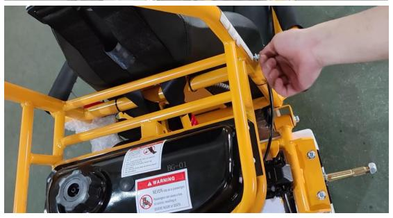
5. Install the rear protective frame fixing pieces, and then tighten the bolts on rear shock absorber as well.
